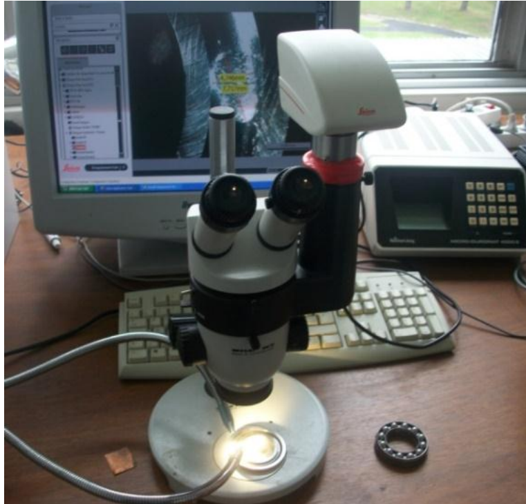
Figure 5. Measurement of the spalling fault size.
