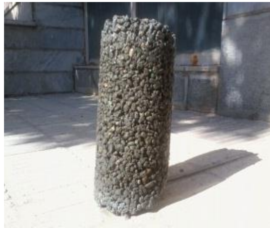
Figure 1. PC Sample for permeability coefficient test.
