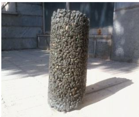
Figure 1. PC Sample for permeability coefficient test.
